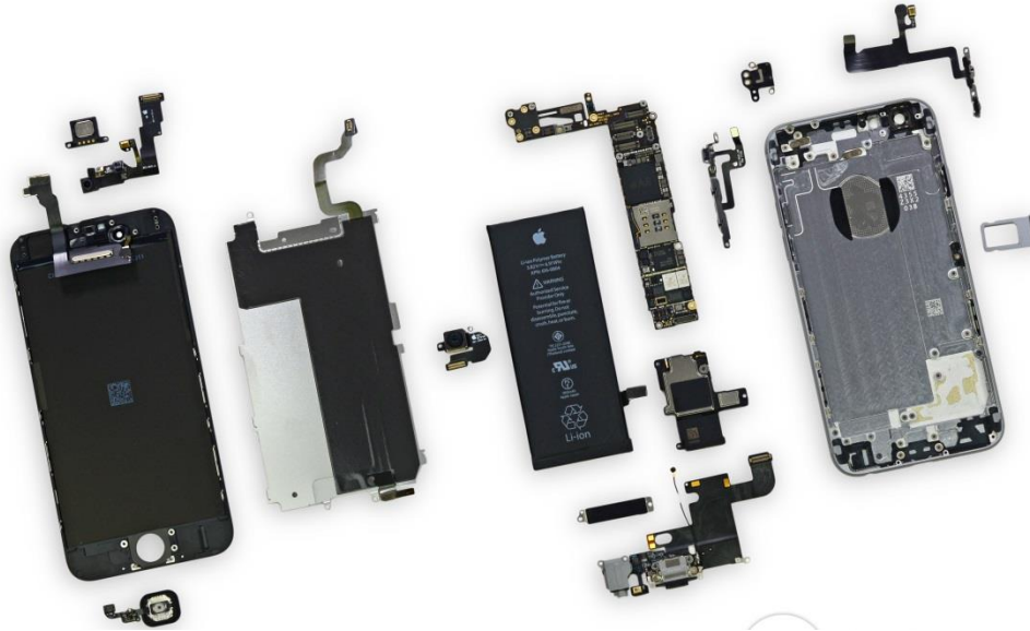
Figure 21: Teardown showing main modules and components of a popular smartphone available in the market in 2016. Source: iFixit
