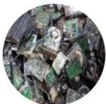
Shredded printed circuit boards (PCB)
